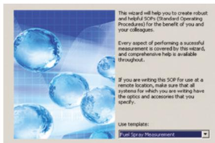
**1** Set up your Standard Operating Procedure (SOP) using the system's integrated method definition wizard. SOPs lock down all aspects of the measurement process including the hardware configuration, analysis settings, triggering options, result parameter reporting and data averaging. Online help supports method specification for different spray types.
