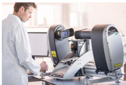
**2** Run the measurement by selecting the desired SOP from the menu system. This automatically configures the system and ensures everything is optimally set to deliver accurate results, including auto-alignment of the optical system. Synchronization of external systems such as extractors, actuators and positioning systems is also supported.
