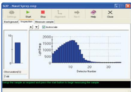
**3** Observe each stage of the measurement via the software's measurement manager. This allows the user to monitor all aspects of the measurement and analysis process. Prompts ensure that the correct sample preparation, handling and disposal procedures are followed.
